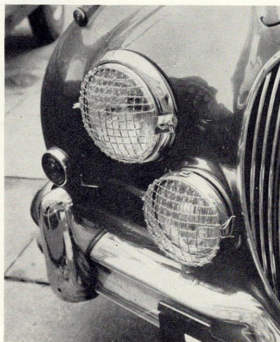
7" Mk. I Stone Guard Spring Clip fitting. Retaining guard to outside of headlamp rim. Car illustrated : Mk. II 3.8 Jaguar, 1963.
